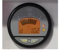
d = hours of operation with diesel engine
