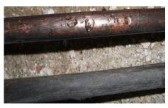
Damaged hydraulic hose pipe
