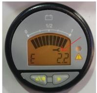
The control unit can store up to 16 alarms which are shown by pressing the right button of the hour counter.
