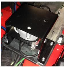
This sensor is connected in parallel to the limit switch that controls that the platform is at a height lower than the transport height (the 12V output signal is interrupted if the platform is lifted above the transport height).
