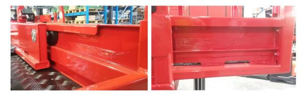
Remove all dirt from the parts before greasing. Use the same grease specified for the runners.
