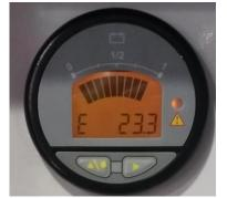
E = hours of operation with electrical engine
