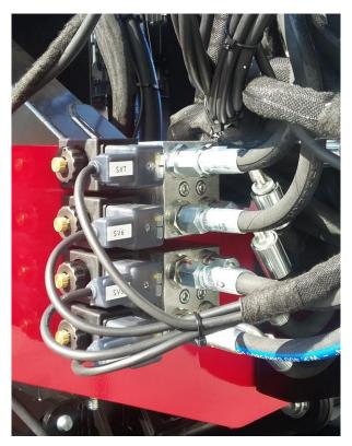
Remove the connectors from the solenoid valves and try to perform manual levelling operations with the machine in the transport position.
