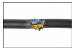
Damaged electric cable
