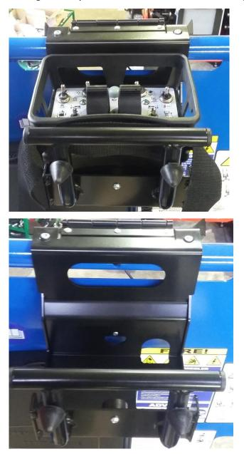
Even the metal support can be removed by unscrewing the special knob.
