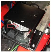
• With the platform in the transport configuration, place the machine with the frame tilted with respect to the horizontal by a value slightly greater than 3° on the lateral. Keep pressed, by inserting a wedge, the limit switch shown in the figure below
