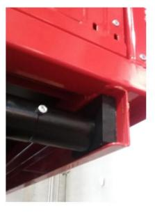
Remove all dirt from the parts before greasing. Use grease type **PAKELO BEARING EP 2** or equivalent.
