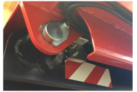
These devices are part of another electromechanical safety ring that prevents the movements of the machine, disabling the outputs of the control unit and disconnecting the other block valves on the levelling cylinders.
