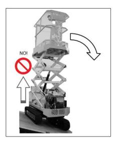
• Avoid smooth, slippery and/or icy surfaces and those covered with sand: they could cause a risk of sliding or tipping during levelling.
